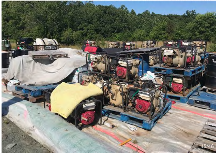
Figure 3: Laydown Yard 046 – Secondary containment structures in place and functioning properly.
