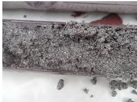
View of ore encountered at 17'-19' bgs during advancement of test boring MW-25.
