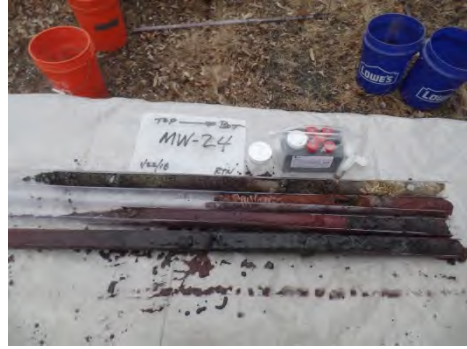
View of soil cores generated during advancement of test boring MW-24.
