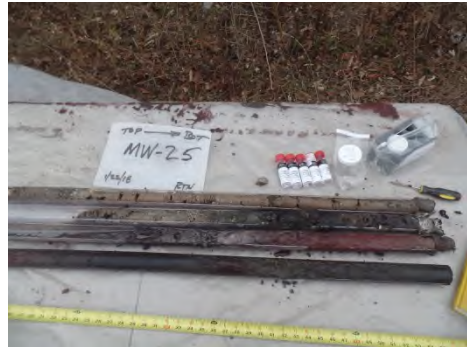
View of soil cores generated during advancement of test boring MW-25.
