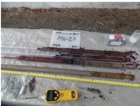
View of soil cores generated during advancement of test boring MW-23.
