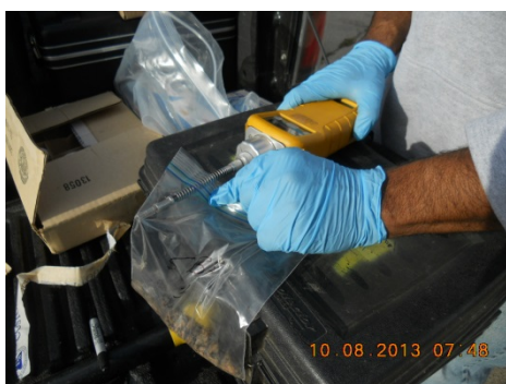
View of soil being screened with a PID.
