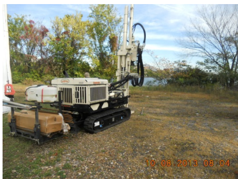
View of direct-push sampling rig during advancement of test boring ICOR-SB4.
