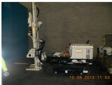
View of direct-push sampling rig during advancement of test boring ICOR-SB12.
