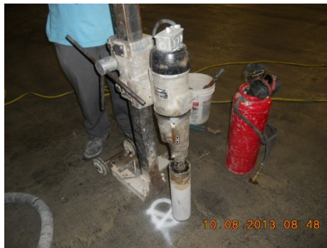
View of coring machine used to core a hole through concrete floor within warehouses.
