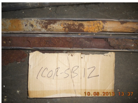
View of intermixed cinder and brick encountered during advancement of test boring ICOR-SB12.
