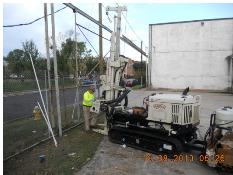
View of direct-push sampling rig during advancement of test boring ICOR-SB1.
