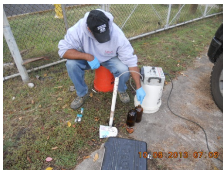
View of groundwater sample being collected from temporary well installed at location ICOR-SB3.
