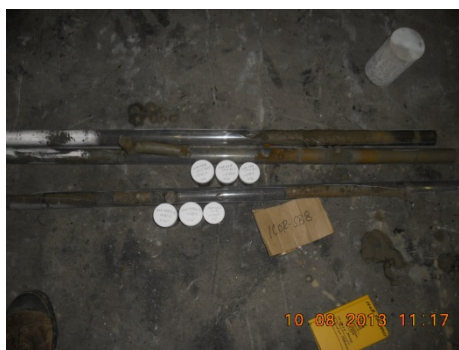
View of soil samples collected for laboratory analysis from cores generated during advancement of test boring ICOR-SB8.
