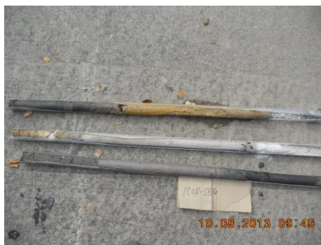
View of sample cores generated during advancement of test boring ICOR-SB6.
