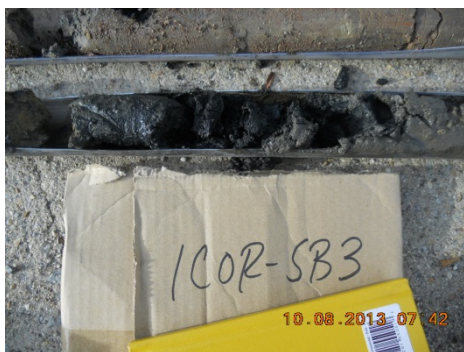
View of oil-stained soil encountered during advancement of test boring ICOR-SB3.
