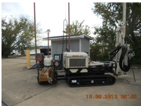
View of direct-push sampling rig during advancement of test boring ICOR-SB2.
