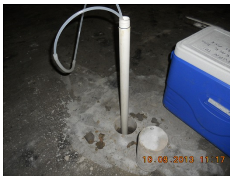
View of temporary well installed at sampling location ICOR-SB8.
