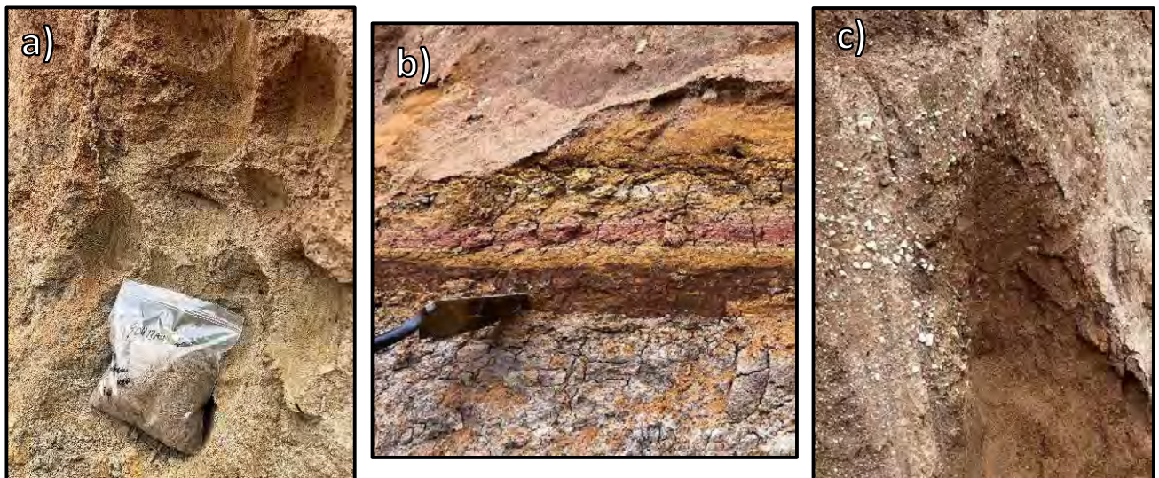
Photographs of samples taken from the smaller, terraced pit area on site 90413AA: a) R-12870, b) image of layers found at site with shovel pointing to an approximately 6" thick paleosol layer, c) R-12871.
