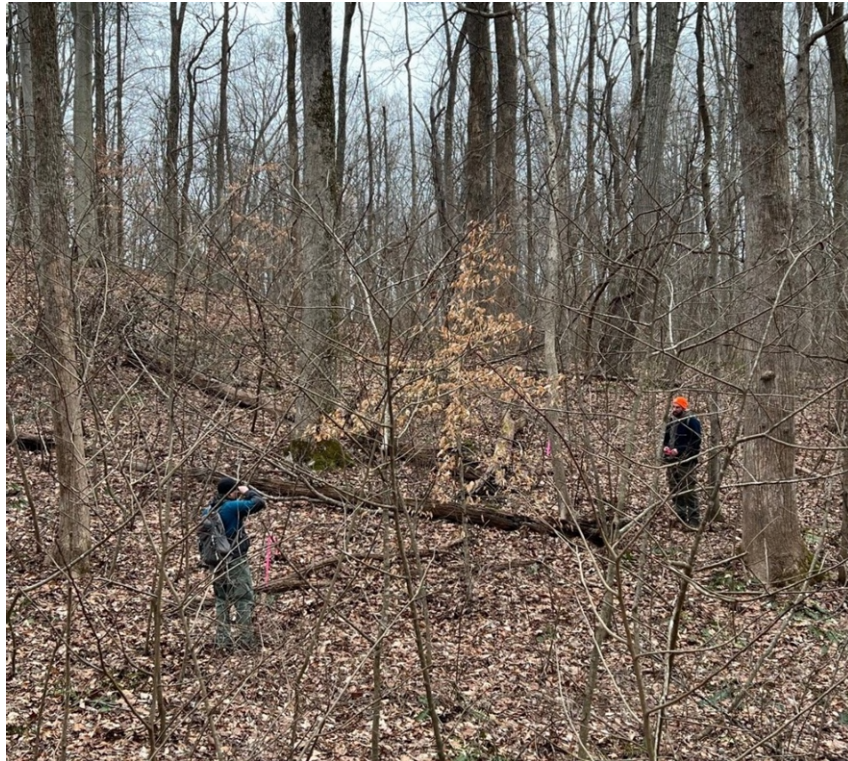
Staff use a clinometer to determine the slope of the proposed trail.
