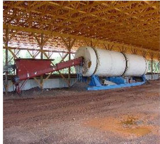
Figure A-14-3. In-Vessel composting is performed in an insulated silo, channel, or bin using a high-rate, controlled aeration system designed to provide optimal conditions. Rotating Drum Composters are a subset of in-vessel composters that aerate compost by turning the compost inside a rotating drum. Photo: Jason Governo, U. of Georgia.
