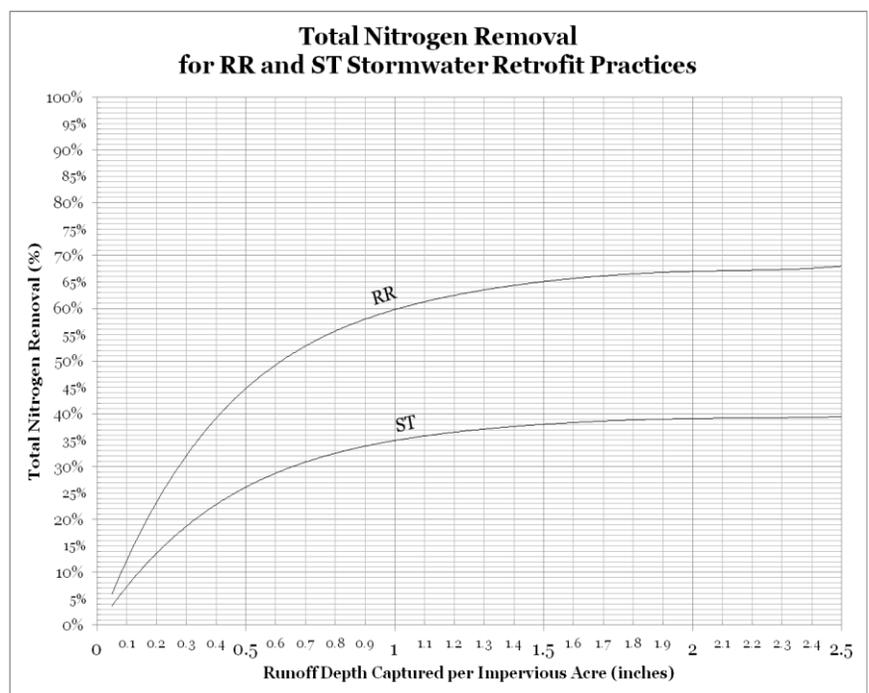
Figure D-1-3. “Adjustor” curves of estimated nitrogen removal for runoff reduction (RR) and stormwater treatment (ST) retrofit practices. Separate curves for phosphorus and sediment are not pictured here but are available in the expert panel report and other resources listed below. Source: Chesapeake Stormwater Network. Use the standard equation for “Runoff Depth Captured per Impervious Acre” (in inches) to find the appropriate location on the X-axis:
