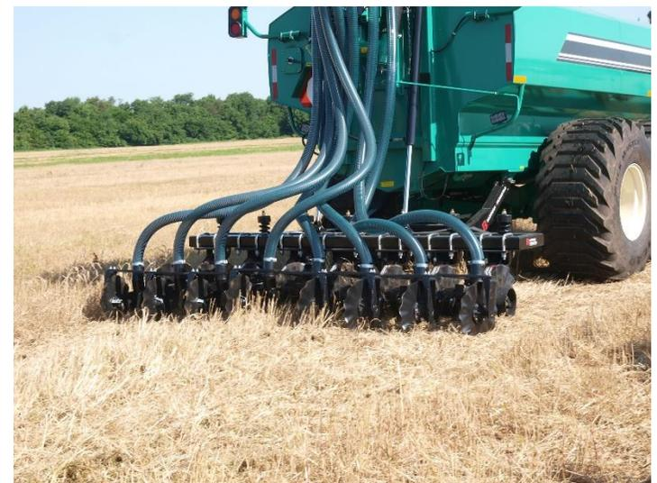
Figure A-17-2. Manure injection mechanically applies the organic nutrients – manure, bio-solids, or compost – into the root zone with surface soil closure at the time of application. This offers the greatest nutrient reduction and odor reduction due to limited soil disruption, amount of material left on the soil and immediate soil closure. Photo: Livestock and Poultry Environmental Learning
