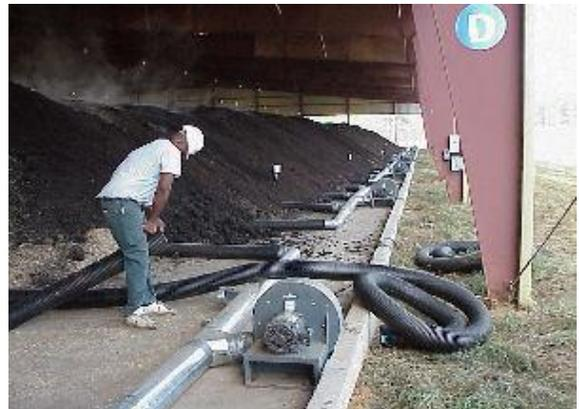
Figure A-14-2. Forced aeration systems, or aerated static piles, use blowers to provide oxygen into the compost pile instead of turning or moving the pile. Photo: Jason Governo, U. of Georgia.
