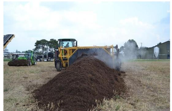
Figure A-14-4. Turned Piles and Windrows rely on frequent turning, usually with specialized machinery, to aerate the compost. Photo: Robb Meinen, Penn State.
