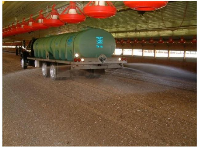
Figure A-20-1. NRCS Practice Code 591: Amendments for the treatment of agricultural waste is the treatment of manure, process wastewater, stormwater runoff from lots or other high intensity areas, and other wastes with chemical or biological additives. Source: NRCS Tennessee ([https://www.nrcs.usda.gov/wps/portal/nrcs/detail/tn/home/?cid=nrcs144p2\\_027179](https://www.nrcs.usda.gov/wps/portal/nrcs/detail/tn/home/?cid=nrcs144p2_027179))
