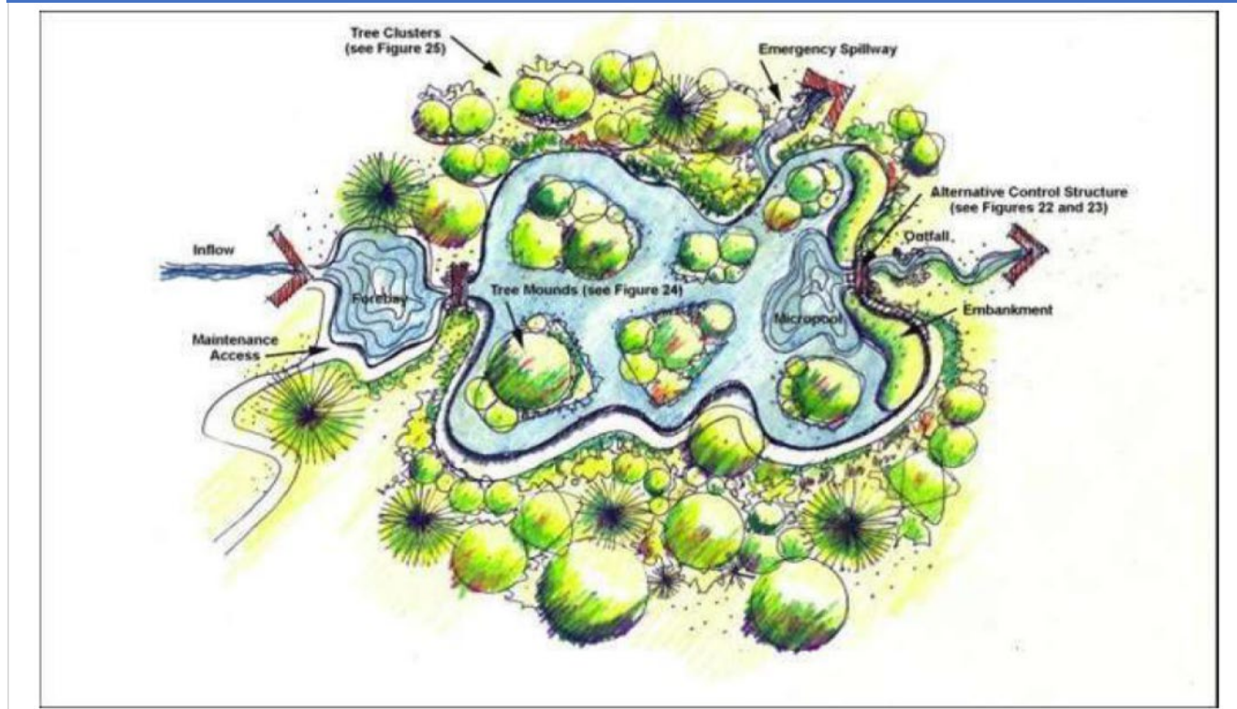
Figure P-BAS-01-1 Constructed Wetland Sketch
