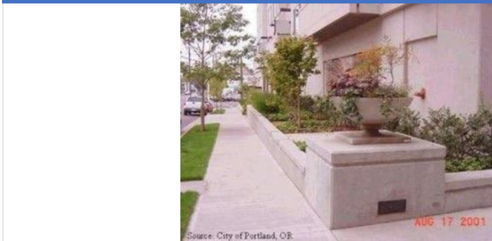
Figure P-FIL-05 B-1 Stormwater planters
