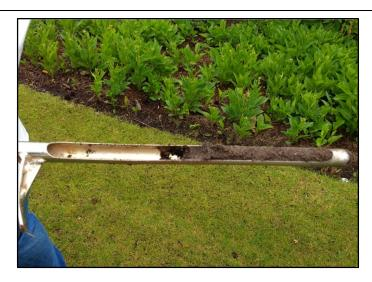
(P-FIL-05) Bioretention media in soil probe Photo credit: DEQ
