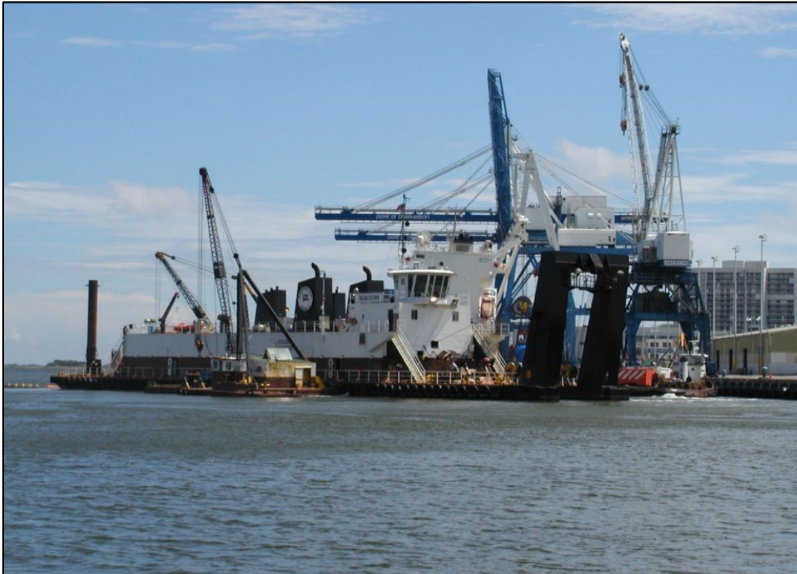
Figure 16: Cutter suction dredger Charleston prepared for maintenance dredging on the upper Delaware River
