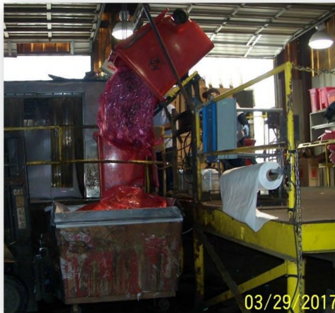
Cart tipping of RMW into autoclave bin
