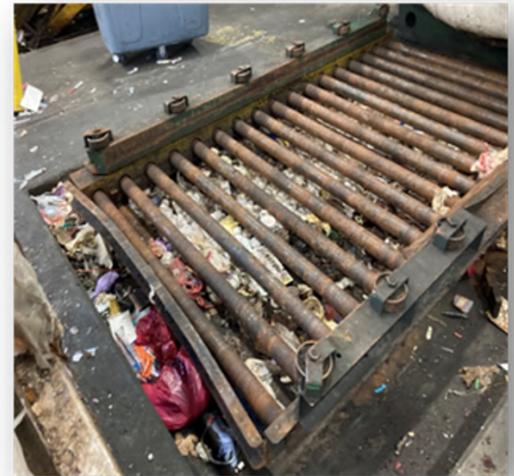
Spilled RMW in autoclave cart lift pit
