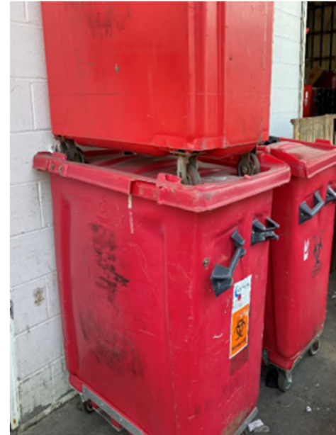
200-gal reusable containers, broken handles & lid locks
