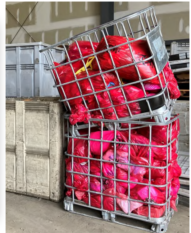
Waste crushed/compressed by stacking of steel cages
