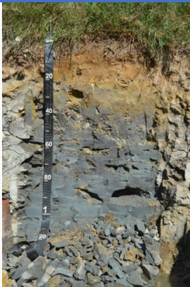
Figure 6-5 Active Acid Sulfate Soil Formed in Cut Coastal Plain Sediments in Stafford County
