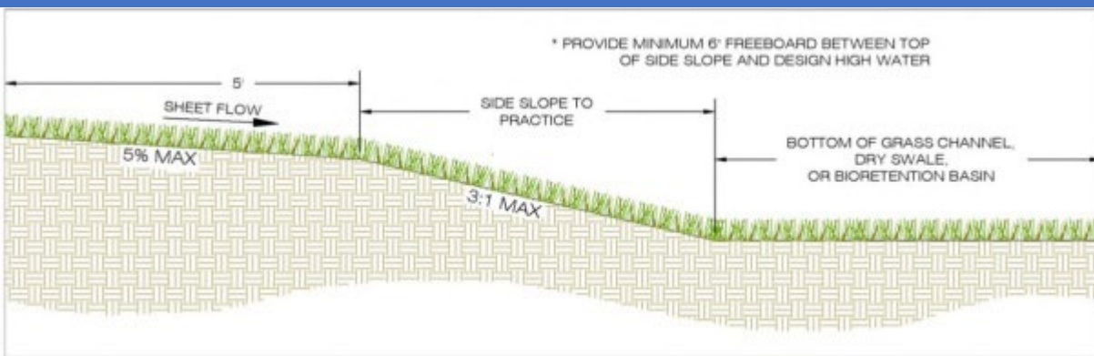
Figure P-CNV-02-7b Pretreatment II – Grass Filter for Sheet Flow
