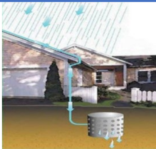
Figure 6-19 Dry Wells Infiltrate Water Into the Ground Instead of Connecting to a Conveyance System
