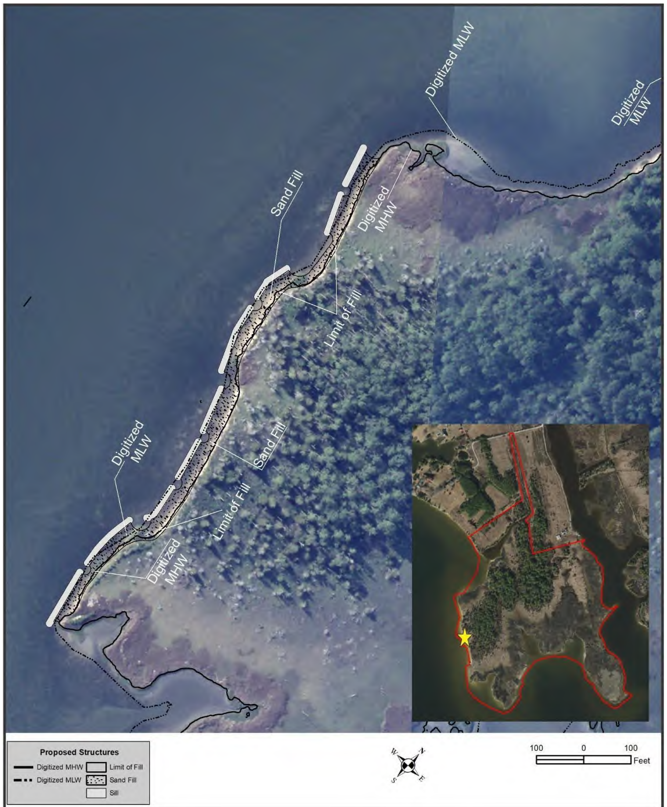
Figure 4-2. Hybrid living shoreline consisting of rock sills, sand fill, and marsh grass plantings. One larger gap was created to allow access.
