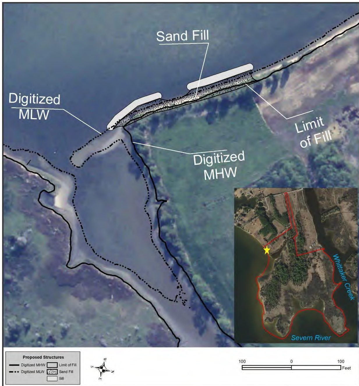
Figure 4-1. Hybrid living shoreline consisting of rock sills, sand fill, and marsh grass plantings. The sills are gapped to allow access.
