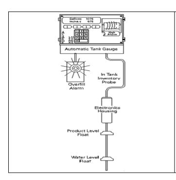
In an Automatic Tank Gauging (ATG) system, a probe installed in the tank is connected to a monitor to provide information on product level and temperature. These systems calculate changes in product volume that can indicate a leaking tank. Each UST must pass at least one 0.2 gallon per hour (GPH) test, once every 30 days.
