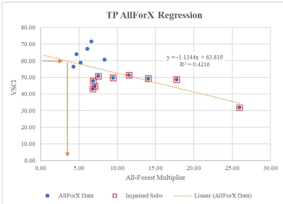
Figure 5-2 Regression between stream condition index and all-forest multiplier for phosphorus in the James River tributaries TMDL using VSCI scores, resulting in an AllForX target value of 3.36.
