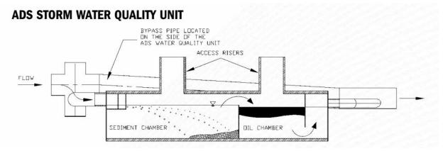
The <u>ADS HDPE Water Quality Unit</u> is designed with two weir plates to trap oils and total suspended solids as the storm water flows through surface drainage structures and into the water quality unit. This structure also incorporates the use of a bypass system, which prevents re–suspension of captured solids by diverting water flows greater than 'first flush'.
