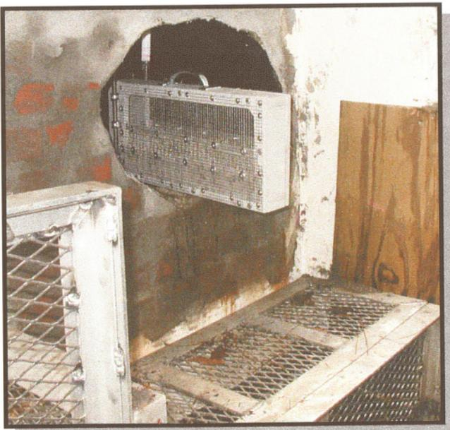
View of sieve sampler in the 30" HDPE outflow pipe.
