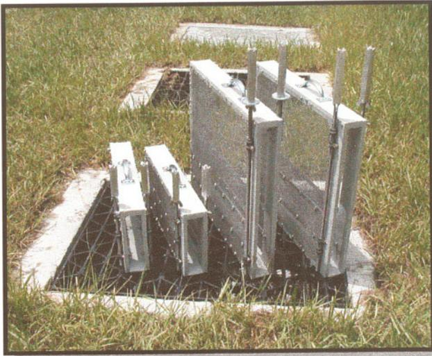
Sieve sampler in the 30" HDPE inflow pipe. The threaded vertical rods on the sides of the samplers adjust to wedge the samplers in the pipe and prevent water flow from dislodging them.
