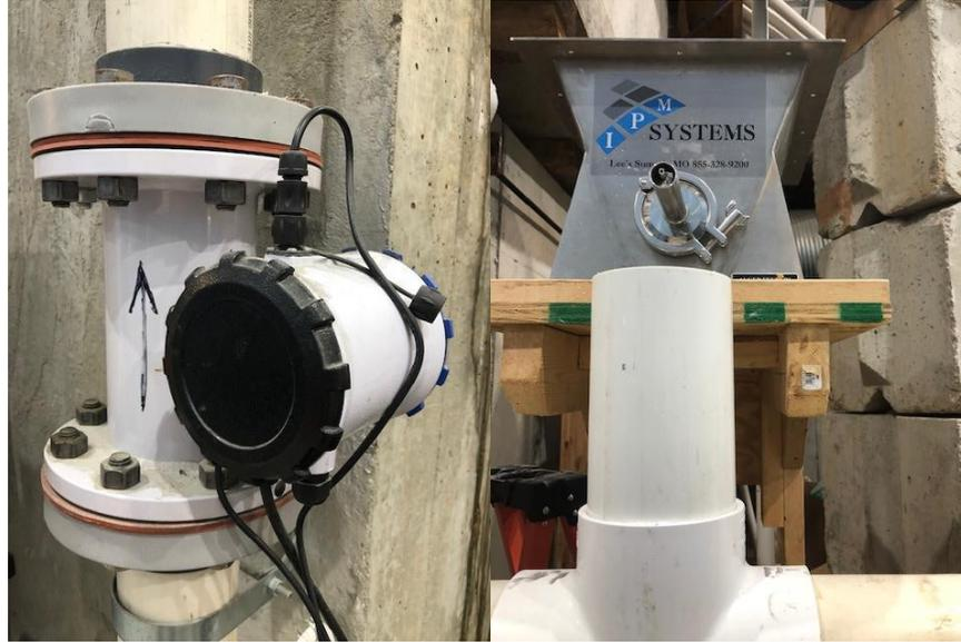
**Figures 4 and 5 Photographs of Flow Meter and Sediment Delivery Port**
