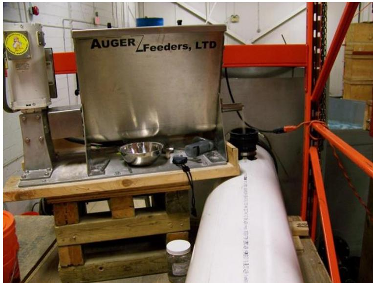
**Figure 7 Sediment Auger Feeder**
