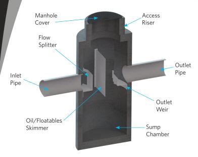
The SciCLONE is manufactured from high density polyethylene components which are non-corrosive and extremely durable.
