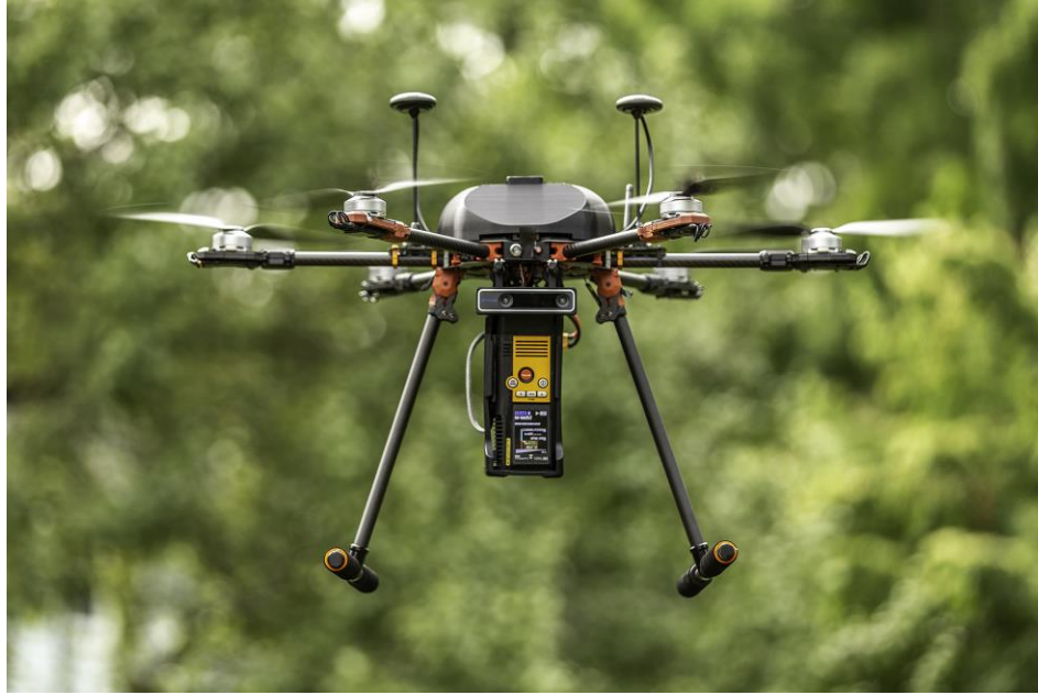
Figure 5:1 Programmable drone with methane sensor (image courtesy of Richard Bishop)
