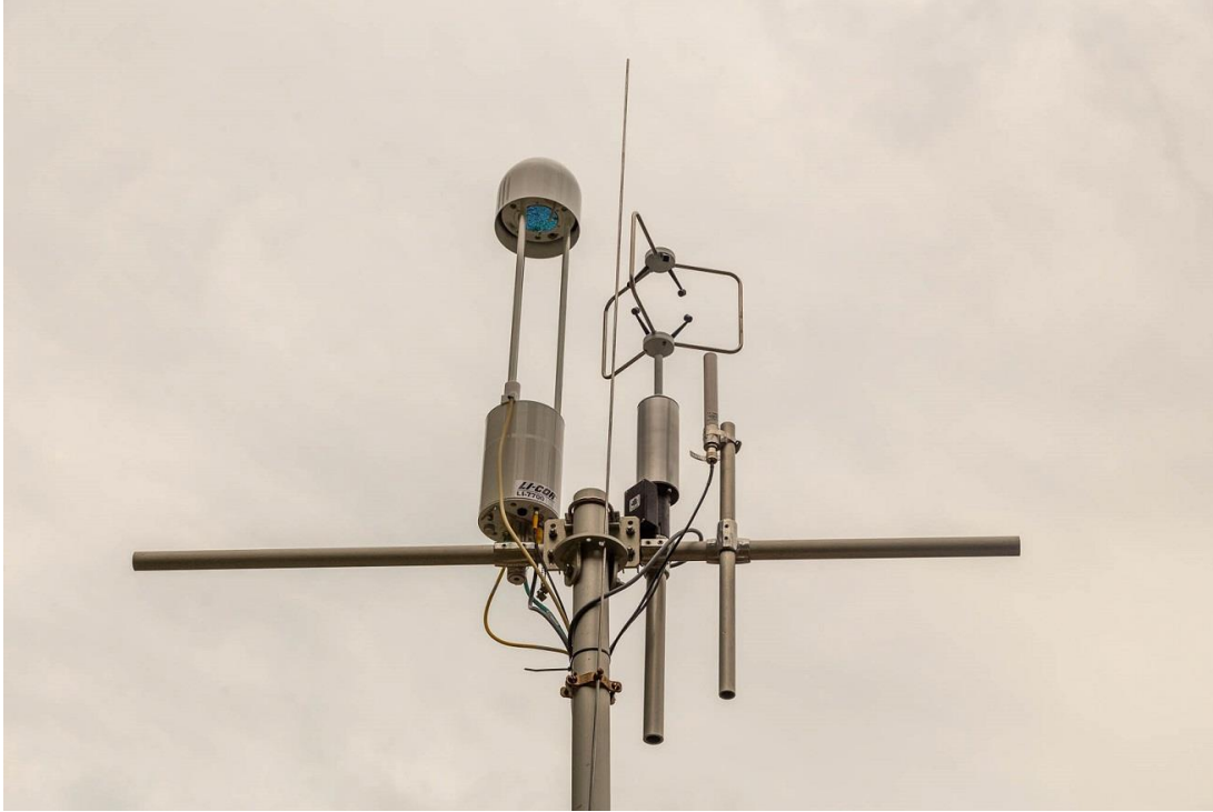
Figure 3:2 Young's Anemometer and LI-7700 in place at Site (image courtesy of Richard Bishop)
