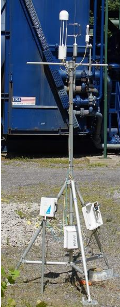
Figure 3:3 Monitoring Station Equipped with, LI-7700,LI-7500A, and Young's Anemometer
