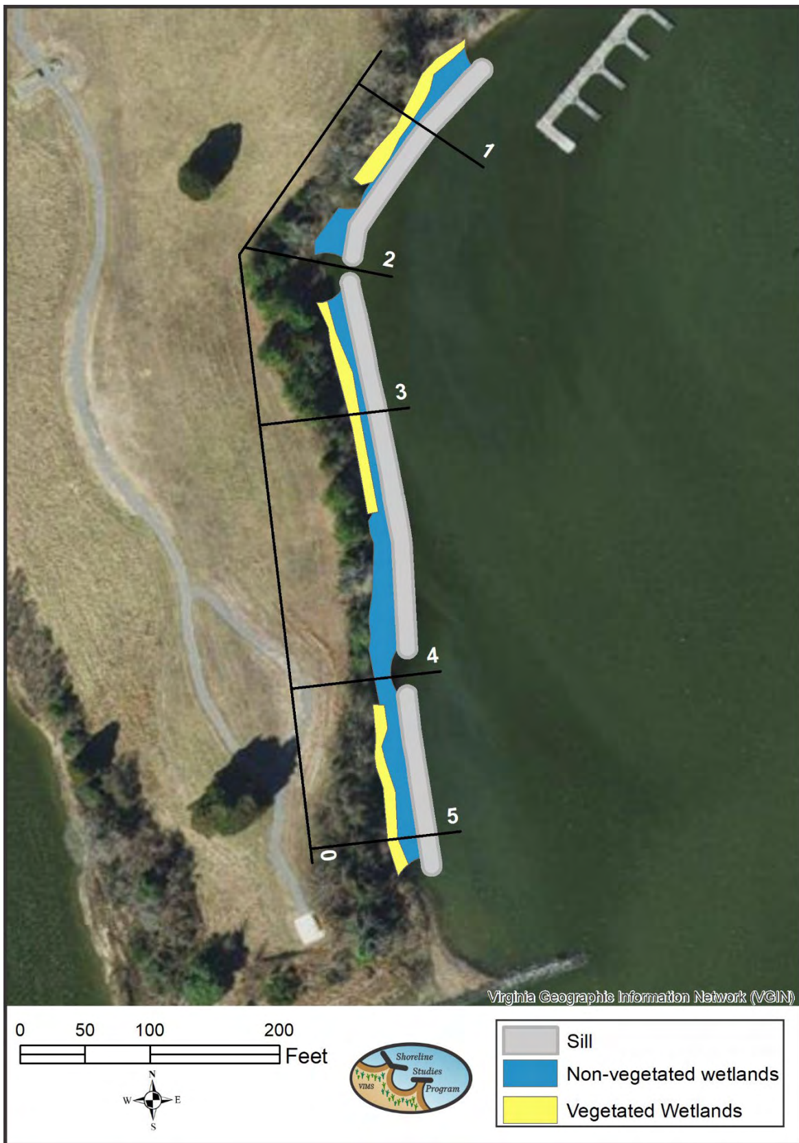
Figure 24. Planform showing the impact of the sand fill on the existing habitats. The shoreline along this reach varies between marsh fringe and no marsh fringe with a scarped, eroding bank.
