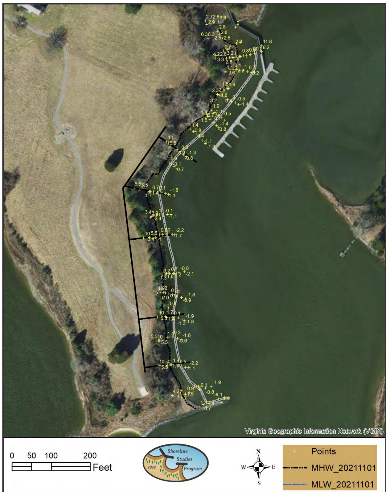
Figure 14. Elevation survey (1 Nov 2021) of the area chosen for the site-specific living shoreline design.
