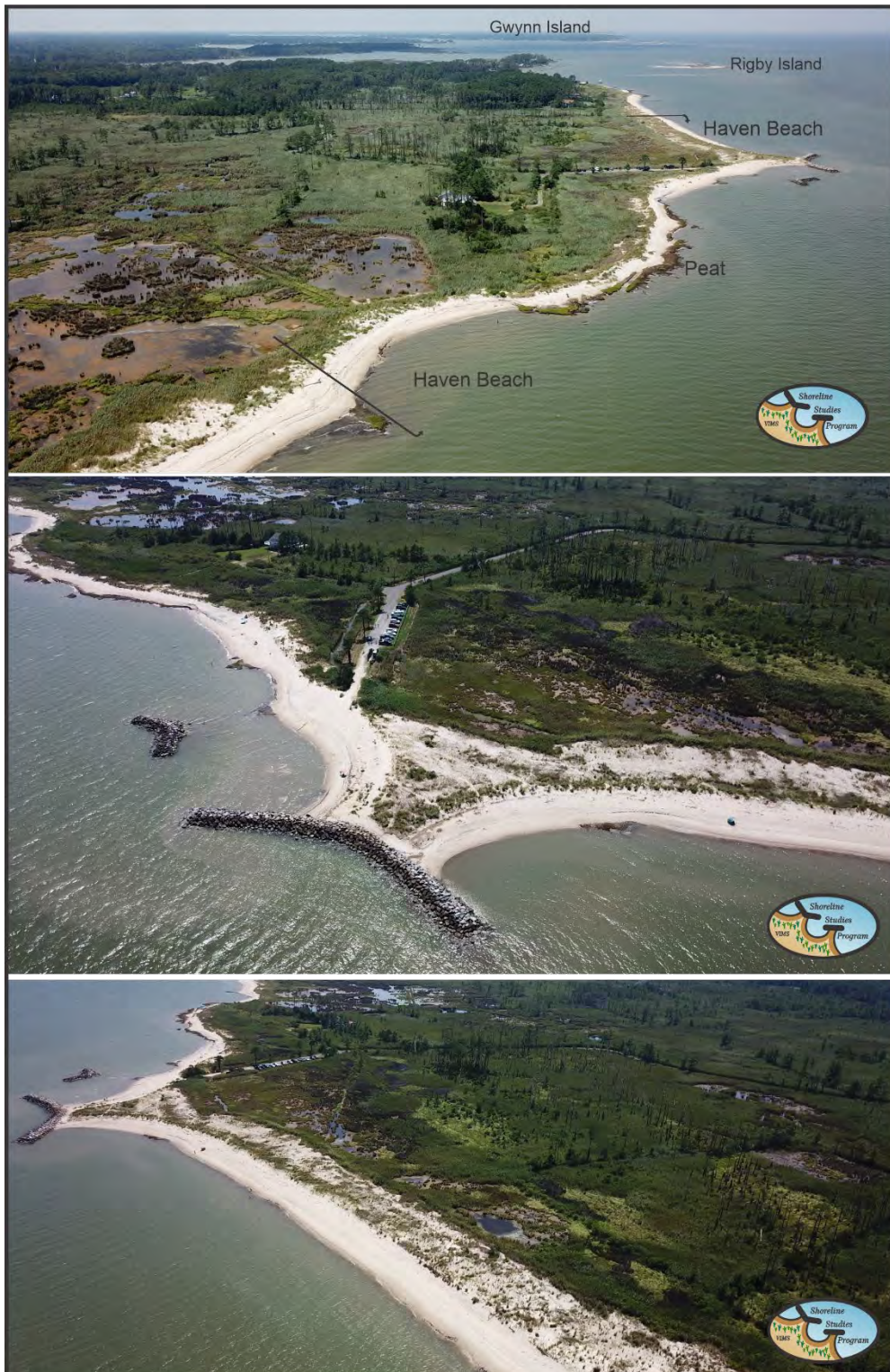
Figure 8-8. Drone imagery taken in July 2020 showing the evolution of Haven Beach. Top: the boundaries Haven Beach are shown. South of the breakwaters, erosion is still occurring and peat is exposed. Middle: The tombolo behind the large breakwater is well-formed with beach and dune vegetation while no sand occurs behind the small breakwater. Top: North of the breakwater, a large beach/dune system has grown since installation of the structures.
