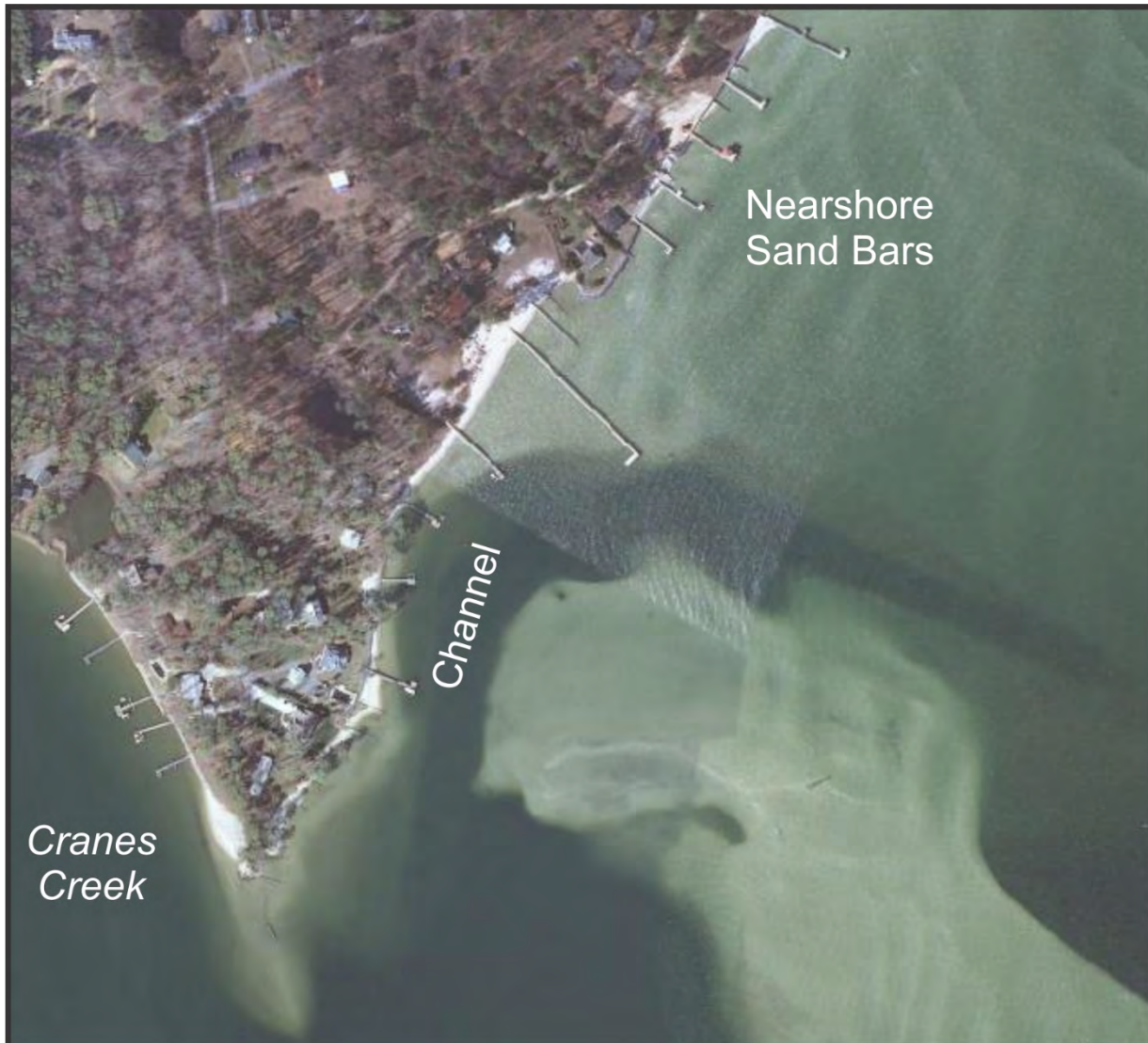
Figure 2-4. A VGIN 2009 photo shows the channel into Cranes Creek in Northumberland County, VA. Sand bars north of the channel will attenuate waves while the shoreline adjacent to the channel has no bars and will feel the full effect of the waves impacting the shoreline.
