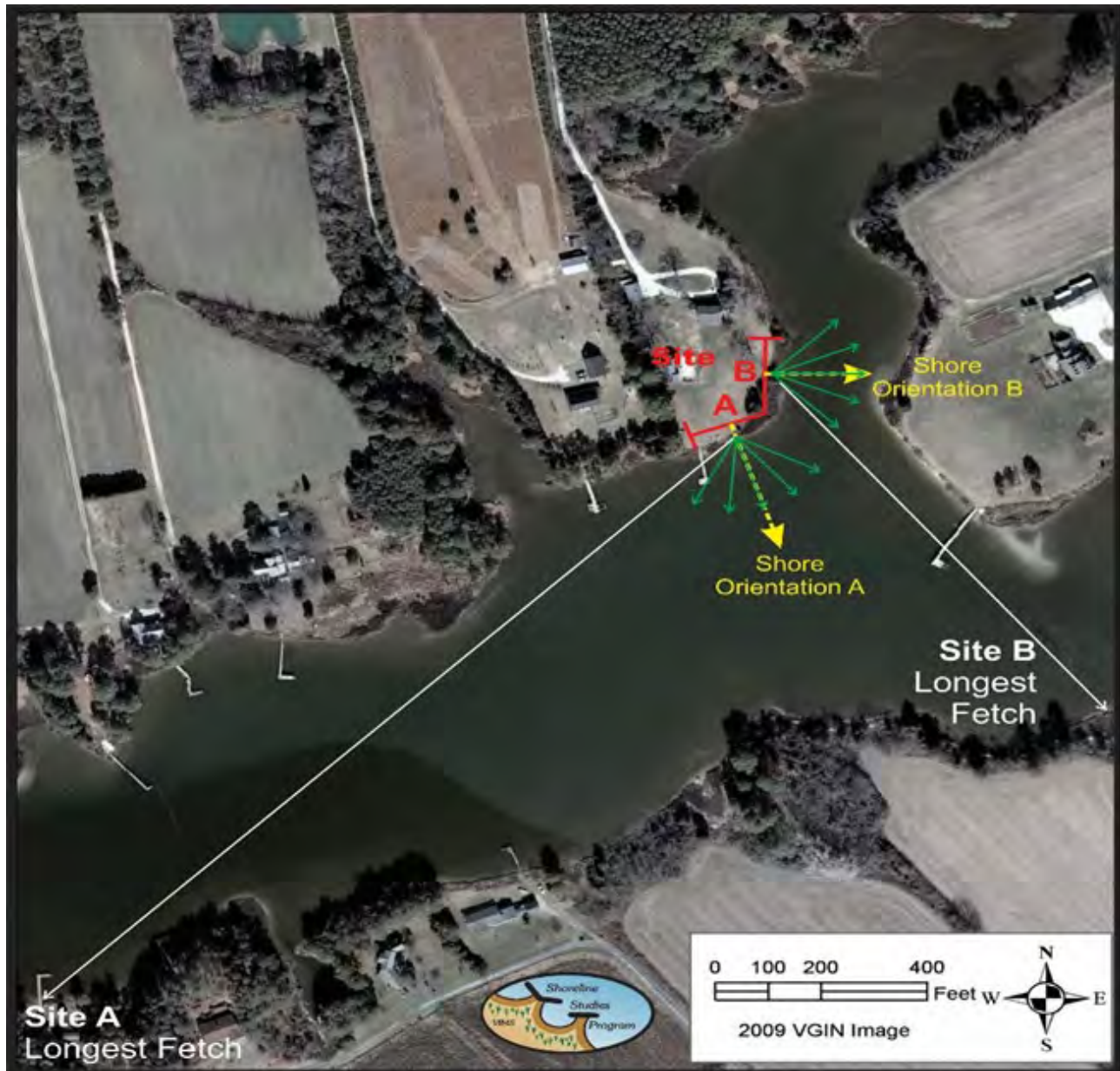
Figure 2-1. Photo depicting the longest fetch for two sections of a site. Section A's shore orientation (direction of face) is southeast while Section B's orientation is east. The green arrows show the vectors measured to determine average fetch while the white arrows show the vector of the longest fetch. Average fetches are measured from the shoreline to the opposite shoreline along the vector line.
