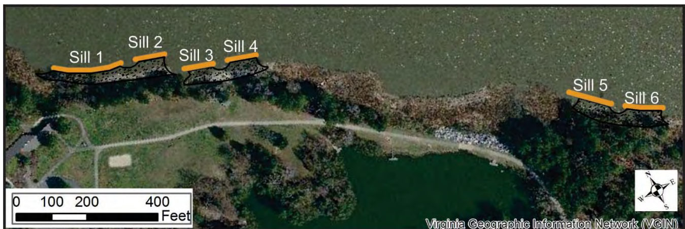
Figure 4-6. Conceptual plan for the living shoreline demonstration project at the York River State Park Visitor's Center. Six sills are recommended along the shoreline to protect the narrow, existing marsh and the eroding upland banks.
