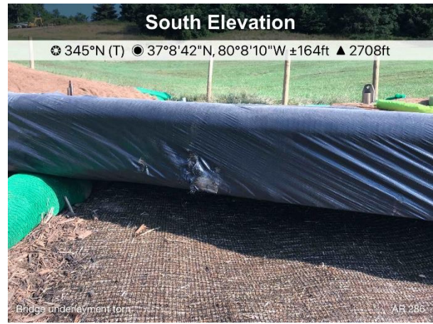
Figure 2: AR 286 bridge underlayment torn
